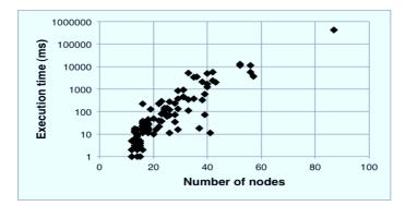
Fig. 11 Computation time of our Tabu algorithm for different size of process models
