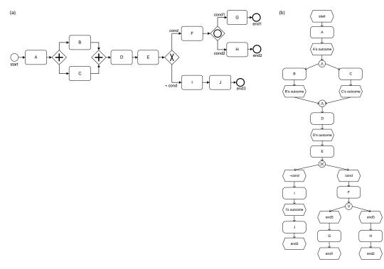
Fig. 18: An example BPMN model (a) and its corresponding model in EPCs (b).
