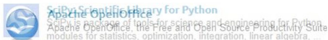
Fig. 2. Difference corresponding to an actual incompatibility (www.sourceforge.net). The text element presented in the baseline is absent in the IUT; instead IUT contains another text.
