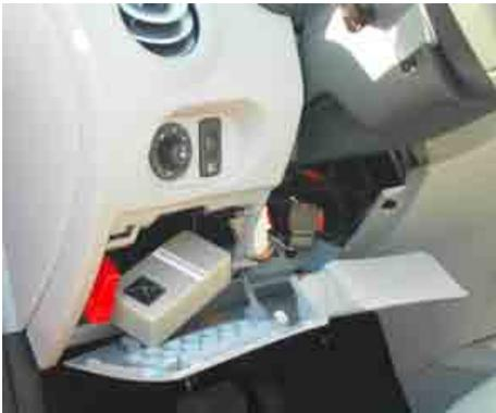
Fig. 2. Embedded GPS System "PUMAS BOX"
