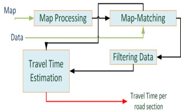
Fig. 4. Overview of the System Architecture
