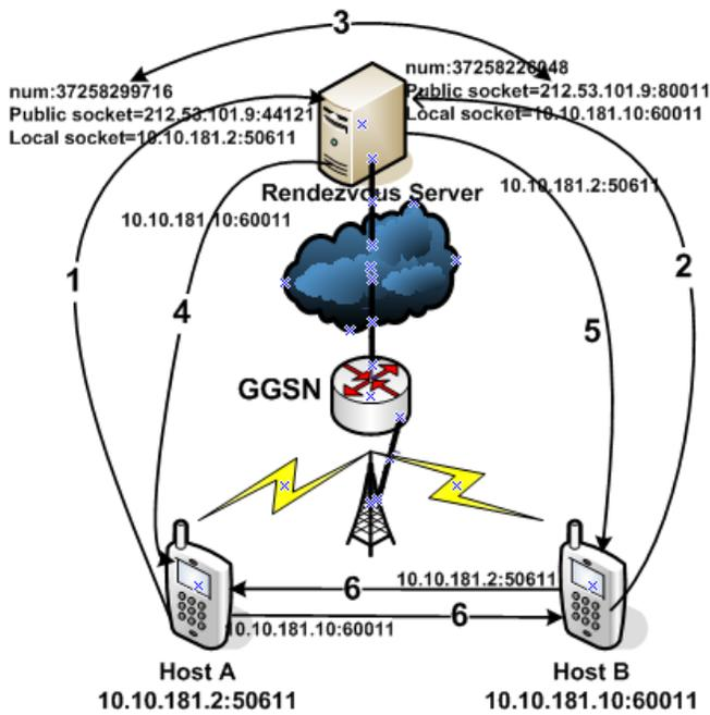
Fig. 9. Establishing connection through hole punching when peers are behind the same NAT
