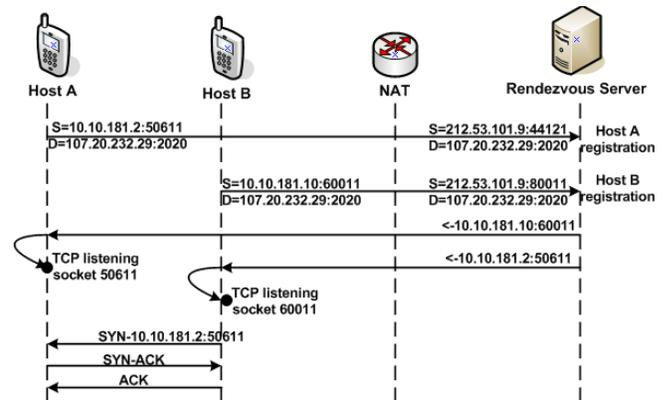
Fig. 10. Sequence diagram showing the timeline of activities performed during the connection establishment between the devices
