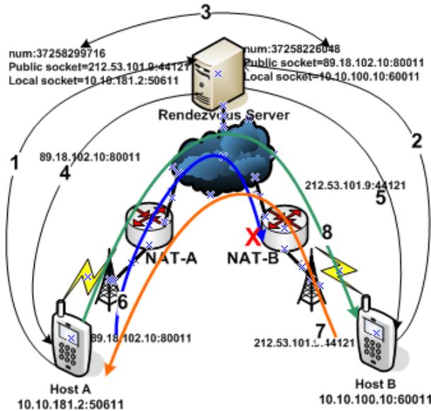
Fig. 11. Establishing connection through hole punching when peers are behind different NATs
