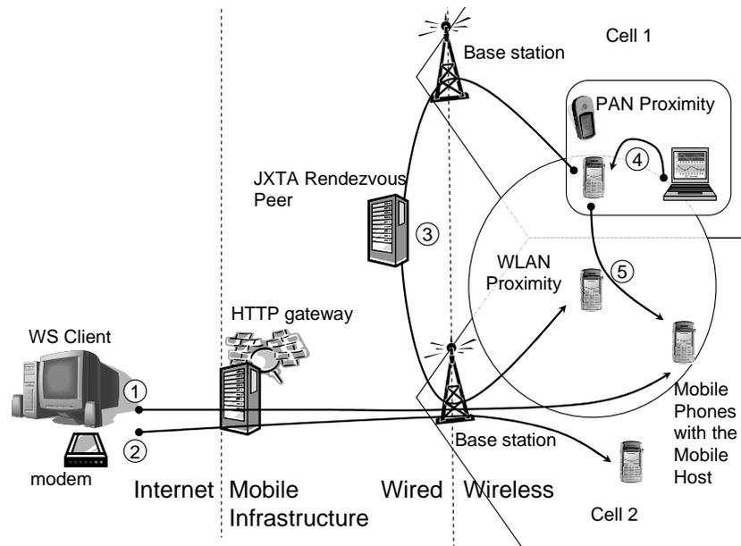
Figure 1: Mobile web service provisioning and interactions
