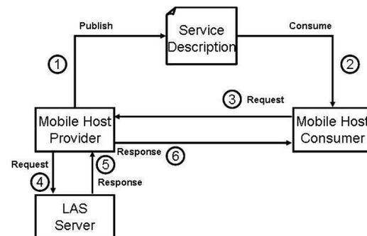
Figure 3. The architecture to access LAS with Mobile Web Services
