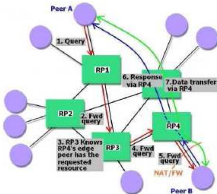
**Figure 5 : Demonstrates the operating principle of JXTA [15].**
