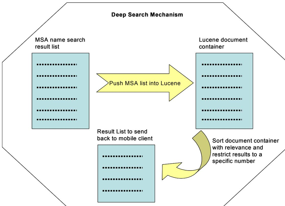
**Figure 29 : Deep Search Mechanism Architecture**
