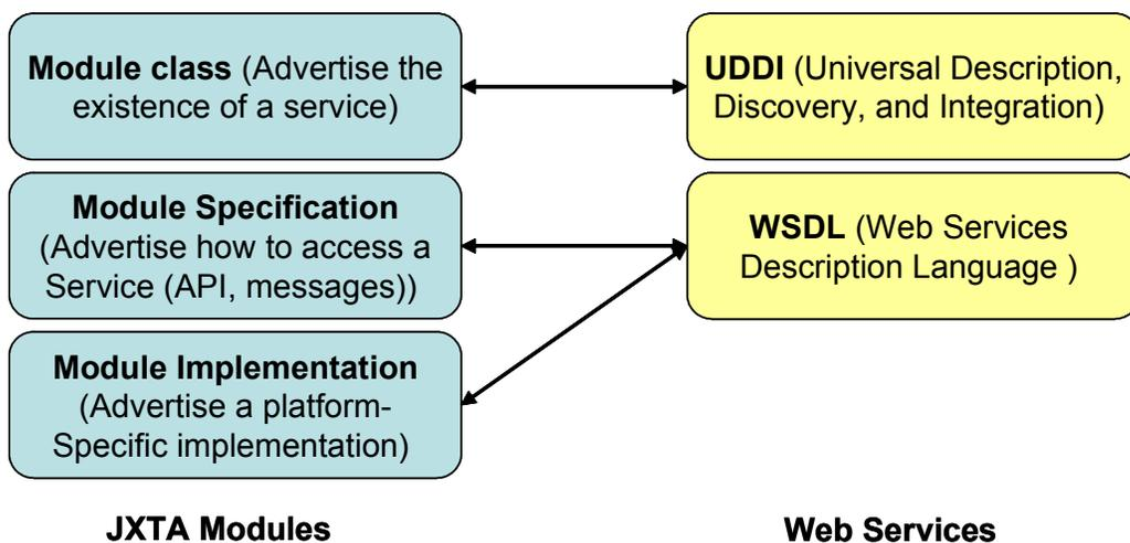
**Figure 17 : Comparison of JXTA Modules and Web Services. The JXTA module together represent a combination of UDDI in the sense of publishing and finding service description and WSDL in the sense of defining transport binding to the service.**
