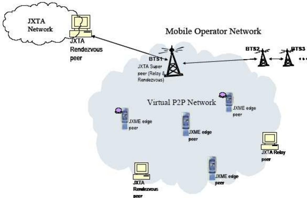
**Figure 22 : General Architecture of Mobile Hosts in JXTA network [43].**
