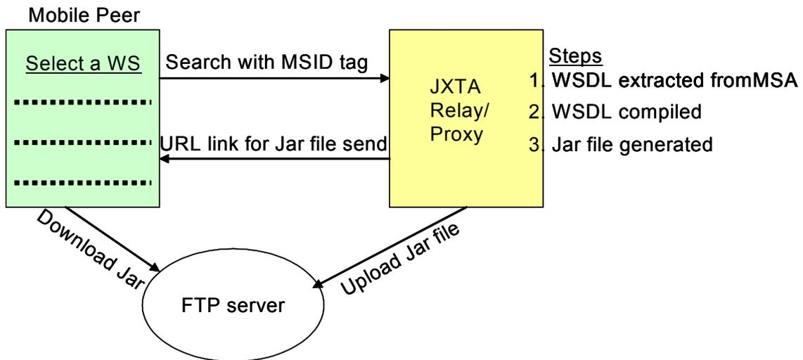
**Figure 30 : Generating and compiling WSDL, and deploying it to a server.**
