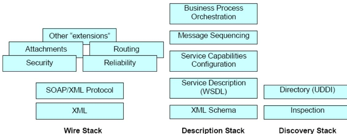
Figure 15 : Web Services Conceptual Architecture (by IBM) [16].
