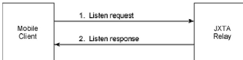
**Figure 35 : The request and response sequence for listening pipe action.**
