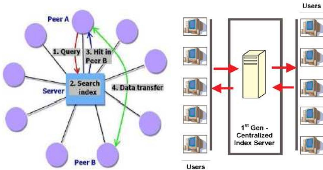
**Figure 3 : Demonstrates the operating principle of Napster and centralized systems [15,20].**
