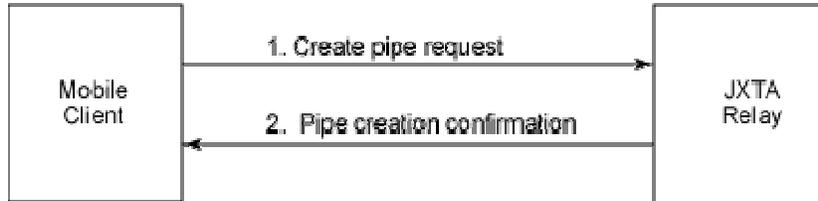
**Figure 34 : A request for creating a pipe and its response**
