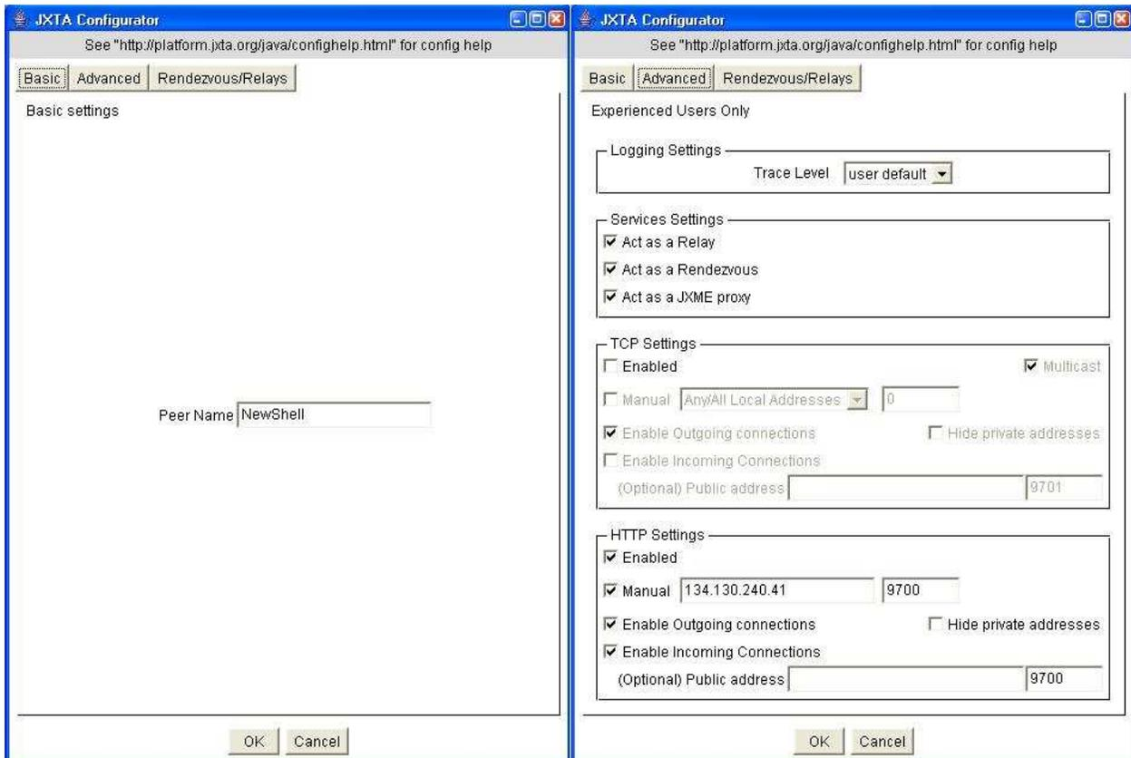
Figure 24 : JXTA Shell configuration screen.
