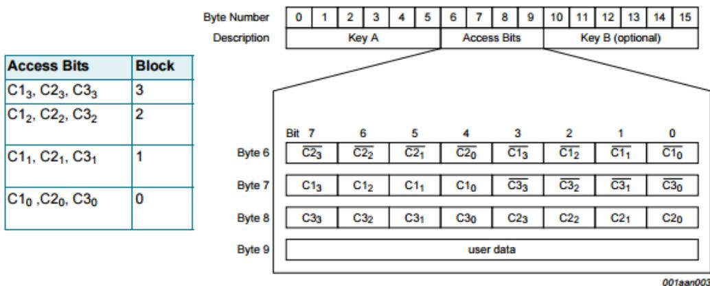
Figure 26. Access conditions for the MIFARE Classic 1K as detailed by sector trailer [[7] Figure 11, Table 6]
