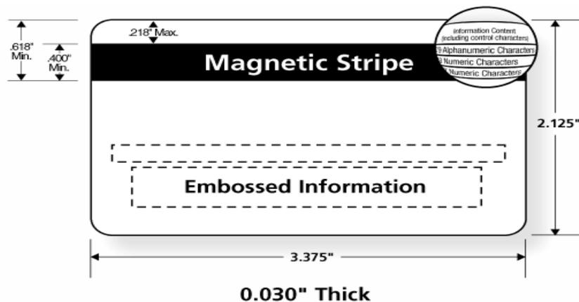
Figure 1. Location of the magnetic stripe on the Magnetic-Stripe Card [2]
