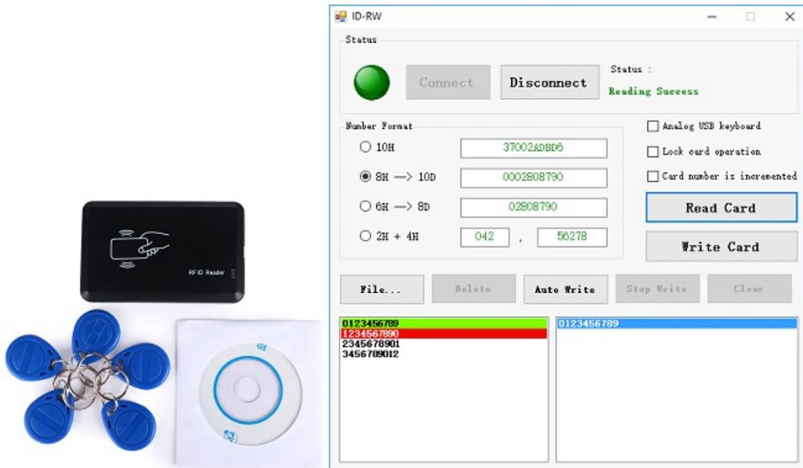
Figure 18. The 125kHz RFID reader/writer/copier and accompanying software and tags
