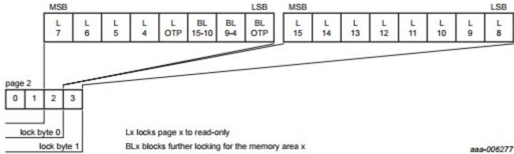
Figure 35. Locking functionality of the lock bytes in page 2 [[4] , Figure 6]
