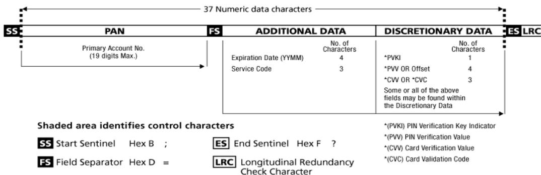
Figure 4. Track 2 Card Data Format for Magnetic-Stripe Cards [2]
