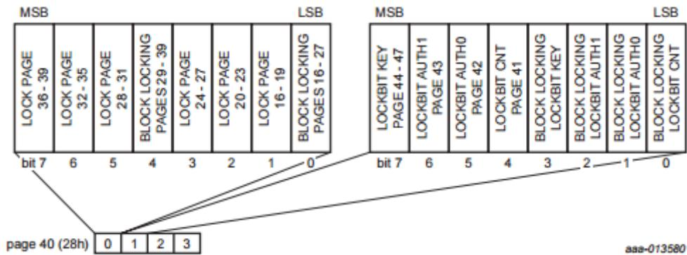
Figure 36. The locking functionality of the lock bytes in page 40 (28h) [[4] , Figure 8]
