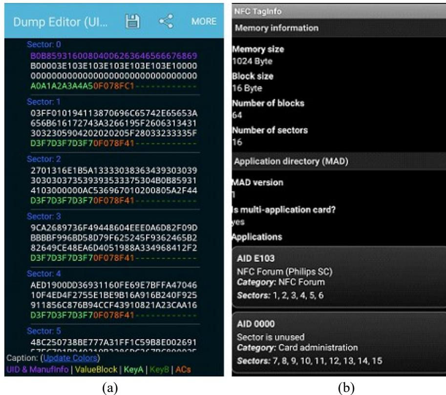
Figure 30. Sections of the output from the MIFARE Classic Tool (a) and NFC TagInfo (b)
