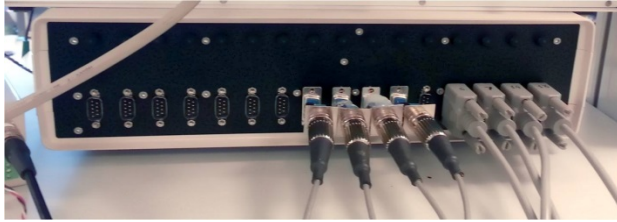
Figure 9. Switchbox with four capacitive and four active electrodes are attached
