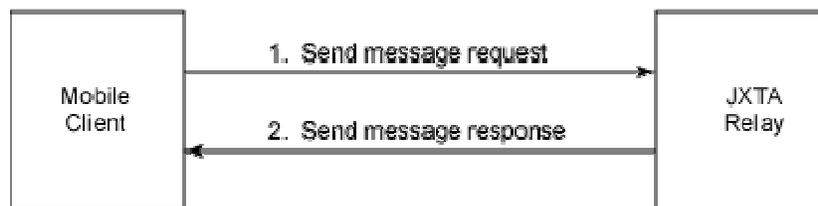
**Figure 36 : Request and response for sending a message over a pipe.**
