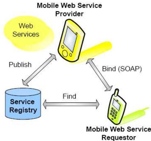
FIGURE 2-16 BASIC ARCHITECTURAL SETUP OF MOBILE HOST [SrJP06A]
