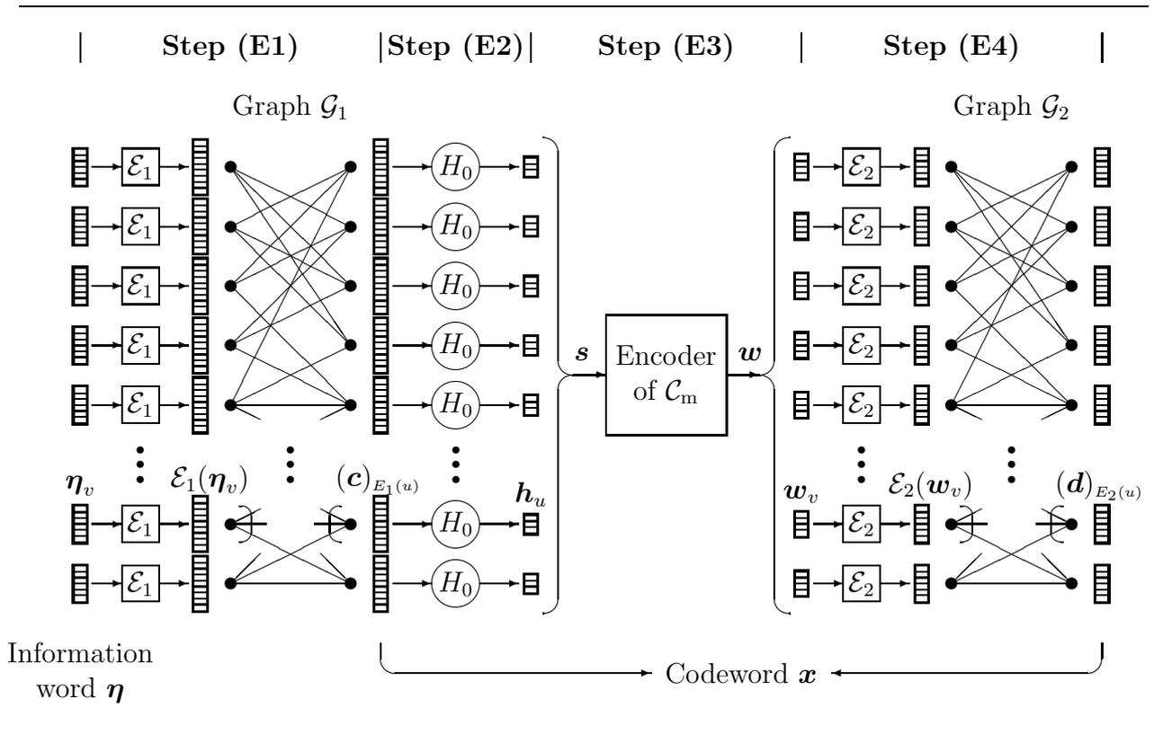
Figure 2.3: Schematic diagram of the encoder for  $\mathcal{C}$ .
